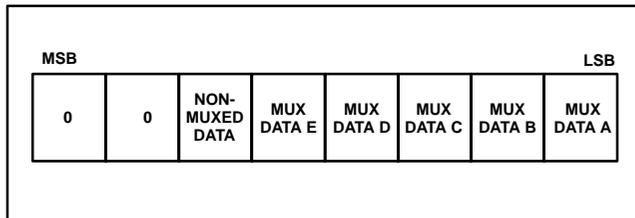
Figure 3. I<sup>2</sup>C Data Byte
