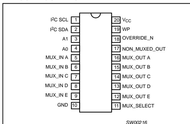
Figure 1. Pin configuration
