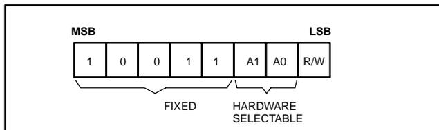
Figure 2. I<sup>2</sup>C Address Byte
