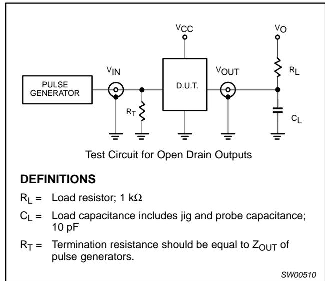
Test Circuit for Open Drain Outputs
