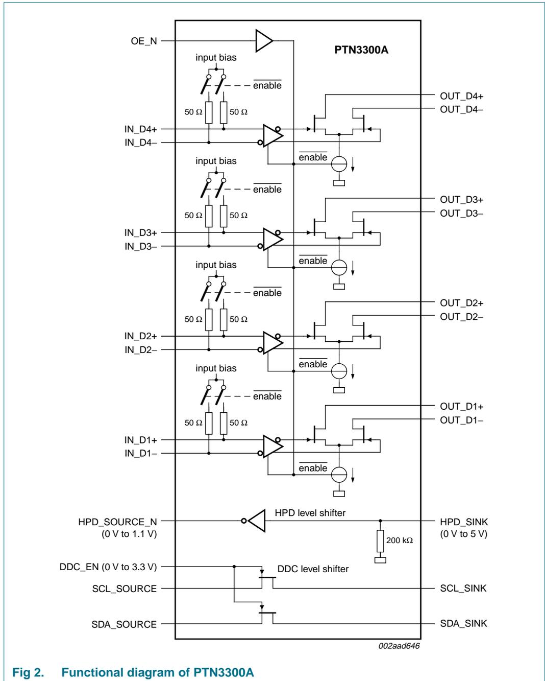
Fig 2. Functional diagram of PTN3300A
