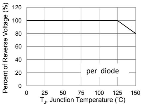
**Fig.5 Operating Temperature Derating Curve**
