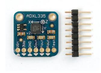
The ADXL335 can measure at least +/- 3G in the X, Y and Z axis. It is perfect for high-resolution static acceleration measurements such as tilt-sensing, as well as for moderate dynamic accelerations from motion, shock or vibration.
