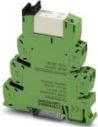
PLC-INTERFACE for railway applications and high continuous currents, consisting of basic terminal block with push-in connection and plug-in miniature relay, range:  $0.7 \times U_N$  to  $1.25 \times U_N$ , temperature class TX:  $-40^\circ\text{C}$  to  $+70^\circ\text{C}$ , 1 PDT, input voltage 24 V DC
