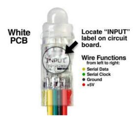
For older bullet pixels with a white circuit board inside, look for the "INPUT" label printed on the board. With this side facing you, the set of wires in front are the input — data arrives here — and the wires underneath are the output to the next pixel.
