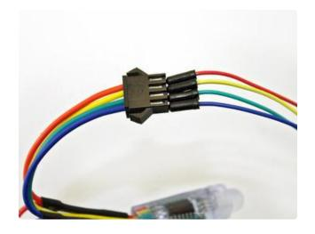
There's one more trick up our sleeve: if you don't have a mating connector available, breadboarding jumper wires can be pressed into the connector - here we're assuming that is the input side!
