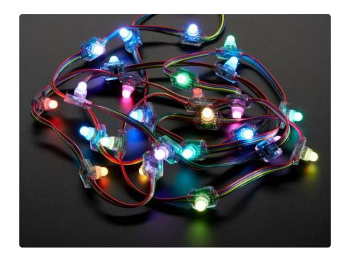
12mm RGB pixels come in two different shapes: "bullet" (thin) and "square" (flat). Both use the same type of LED, driver chip and data protocols...the main difference is how they can be mounted: bullets fit better into narrow spaces, while squares are better suited to shallow spaces.
