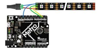
Microcontroller GND to Blue Ground line Microcontroller D3 to Green Serial Clock line
