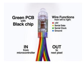
For bullet pixels with a green circuit board inside, look for the rectangular black chip on one side of the board. With this chip facing you, the set of wires in front are the input — data arrives here — and the wires underneath are the output to the next pixel.
