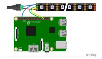
Microcontroller GND to Blue Ground line Microcontroller D6 to Green Serial Clock line
