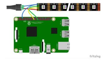
Microcontroller GND to Blue Ground line Microcontroller SCLK to Green Serial Clock line
