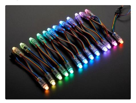
Both types use an 8mm diffused RGB LED ("12mm" refers to the size of the mounting hole for installation) — diffused pixels mix colors nicer. At 5 volts, they draw a maximum of 60 milliamps per pixel: 20 mA each for red, green and blue.
