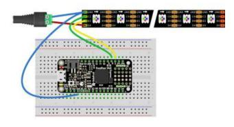
Microcontroller GND to Blue Ground line Microcontroller D6 to Green Serial Clock line
