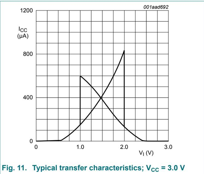
Fig. 11. Typical transfer characteristics;  $V_{CC} = 3.0\text{ V}$
