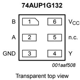
Fig. 6. Pin configuration SOT891, SOT1115 and SOT1202 (XSON6)
