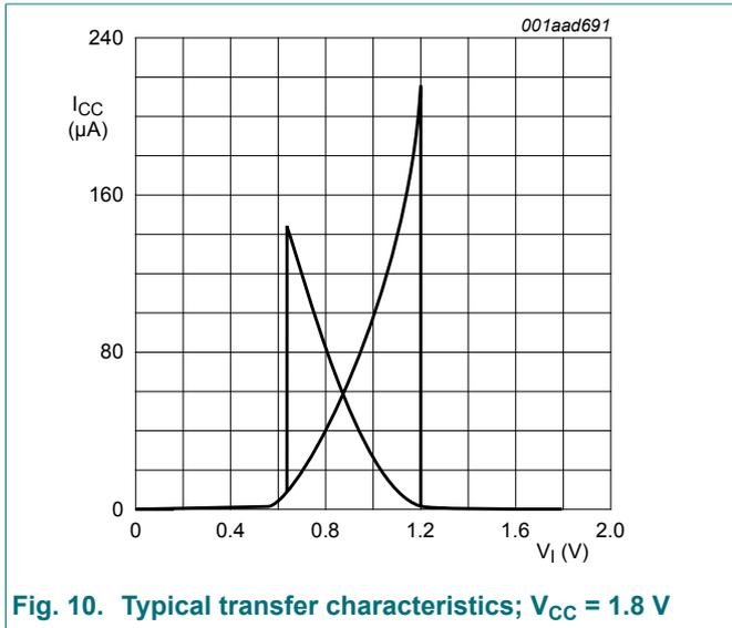
Fig. 10. Typical transfer characteristics;  $V_{CC} = 1.8\text{ V}$
