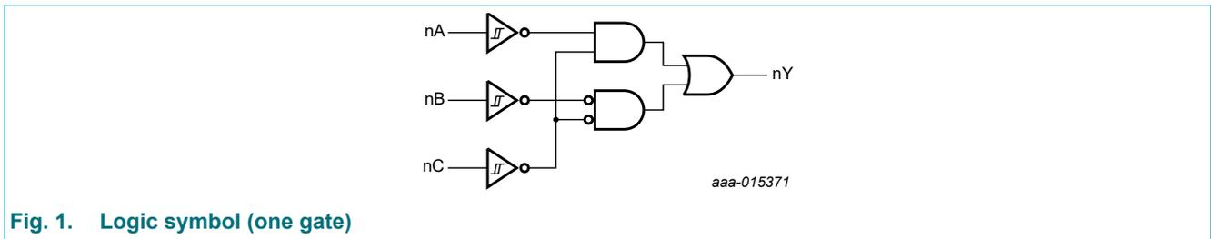
Fig. 1. Logic symbol (one gate)
