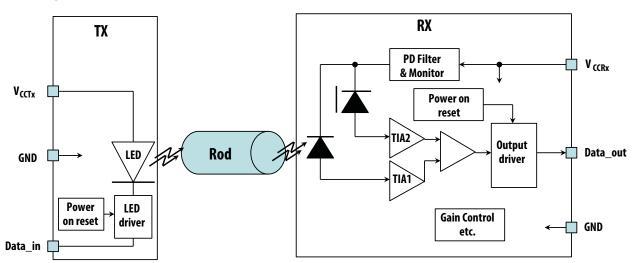
A low Input signal at Data\_in results in a low output signal at Data\_out (non-inverted Tx to non-inverted Rx).
