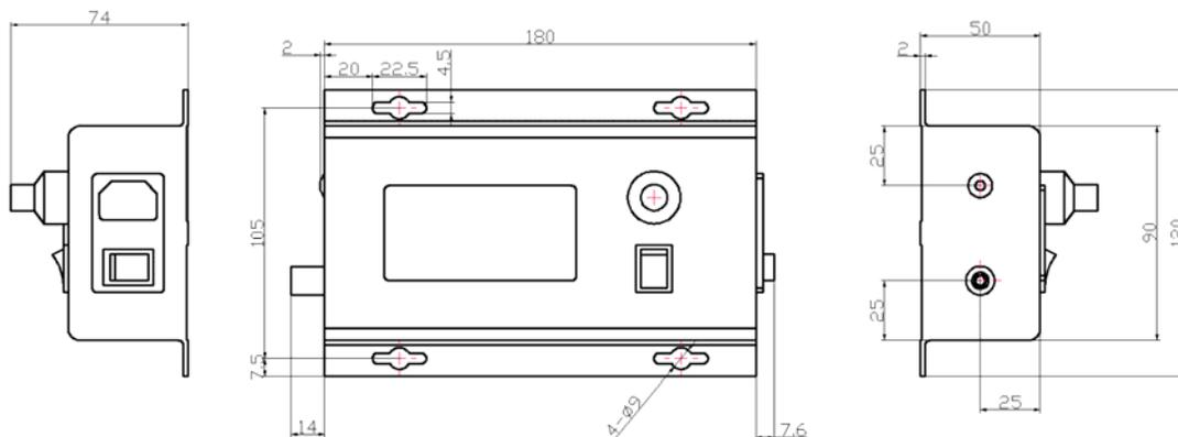
Figure 9. Dimensions for AHVAC10KVR5MABT
