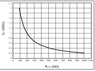
Figure 2 Operating Frequency vs. R<sub>TON</sub> Resistance
