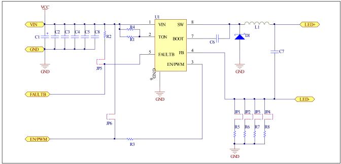
Figure 4: IS31LT3954A/IS32LT3954A Demo Board Schematic
