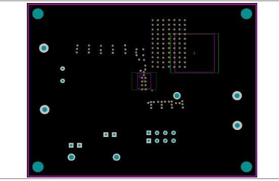
Figure 7: Board Component Placement Guide - Bottom Layer
