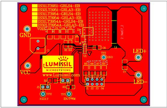
Figure 6: Board PCB Layout - Top Layer
