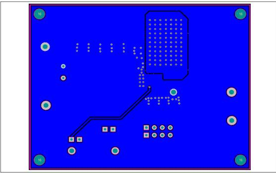
Figure 8: Board PCB Layout - Bottom Layer
