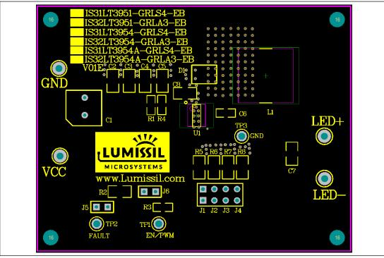
Figure 5: Board Component Placement Guide - Top Layer
