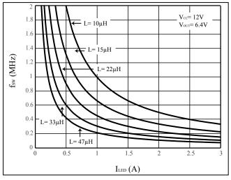
Figure 3 Inductance Selection Based On 30% Current Ripple
