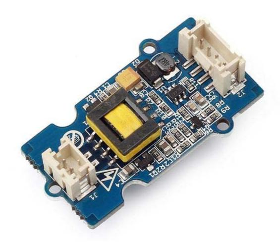
Grove - EL Driver is designed for driving EL Wires. It integrates a very small inverter to drive the EL Wire, so you can easily light up the EL Wire with just one single Grove cable.
