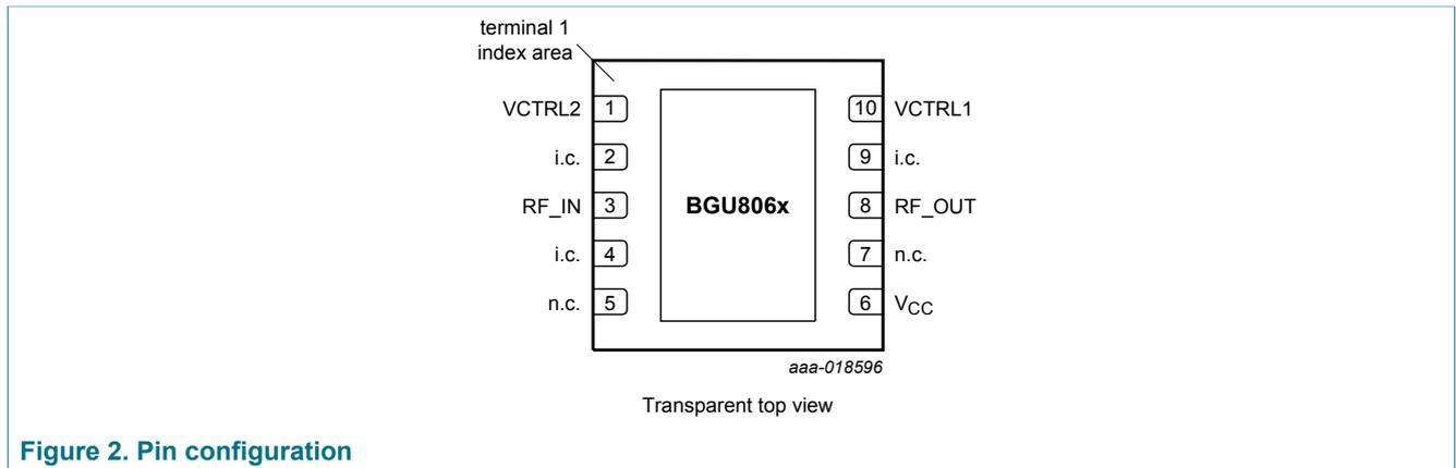
Figure 2. Pin configuration
