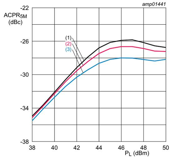
$V_{DS} = 30\text{ V}; I_{Dq} = 300\text{ mA}; V_{GS(amp)peak} = 1.3\text{ V}.$
