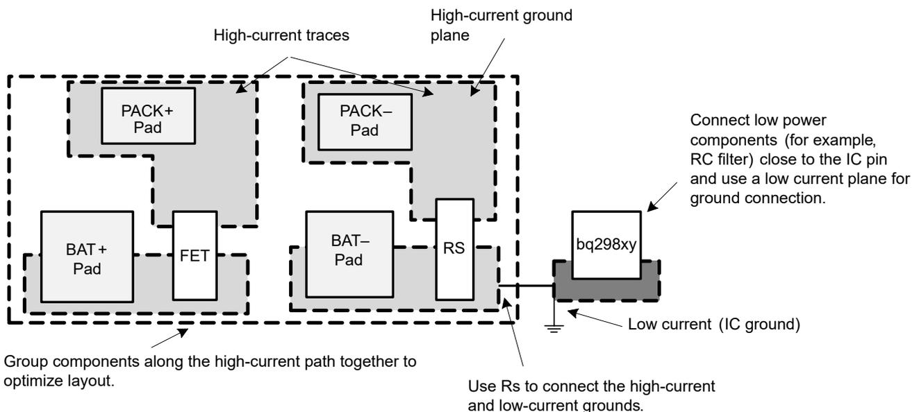
Figure 11-1. Component Placement and Grounding Pattern Example
