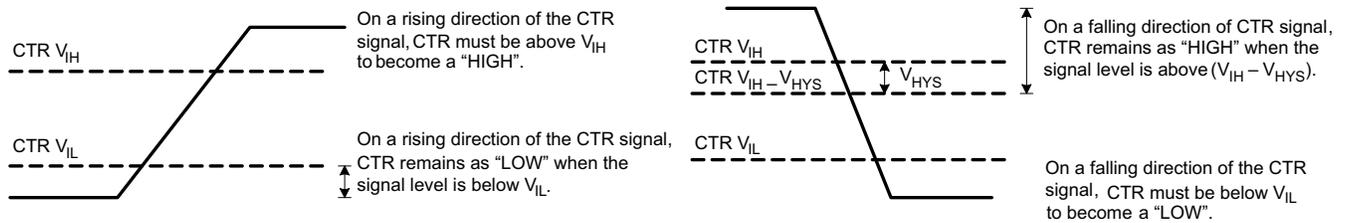
**Figure 8-1. CTR Level in Rising and Falling Direction**
