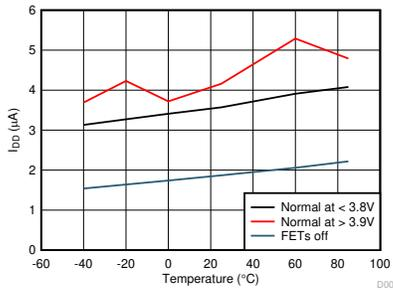
**Figure 7-1. Normal and FET Off Current Across Temperature**
