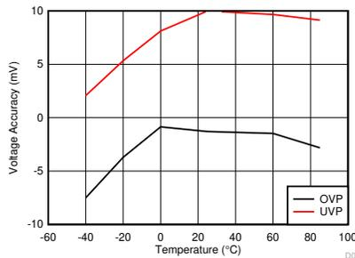
**Figure 7-3. Overvoltage and Undervoltage Accuracy Across Temperature**
