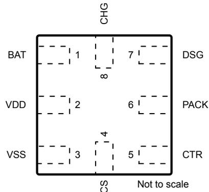
Figure 6-1. RUG Package 8-Pin X2QFN Top View
