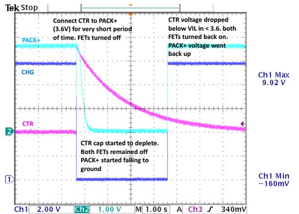
**Figure 9-11. Setup CTR for System Reset (Using 5 M $\Omega$  and 1  $\mu F$  RC)**
