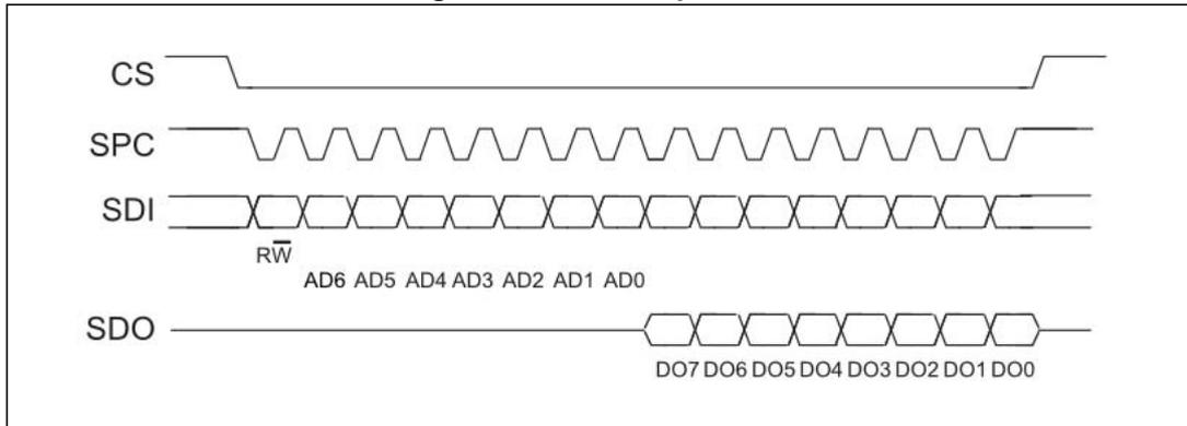
The SPI read command is performed with 16 clock pulses. The multiple byte read command is performed by adding blocks of 8 clock pulses to the previous one.
