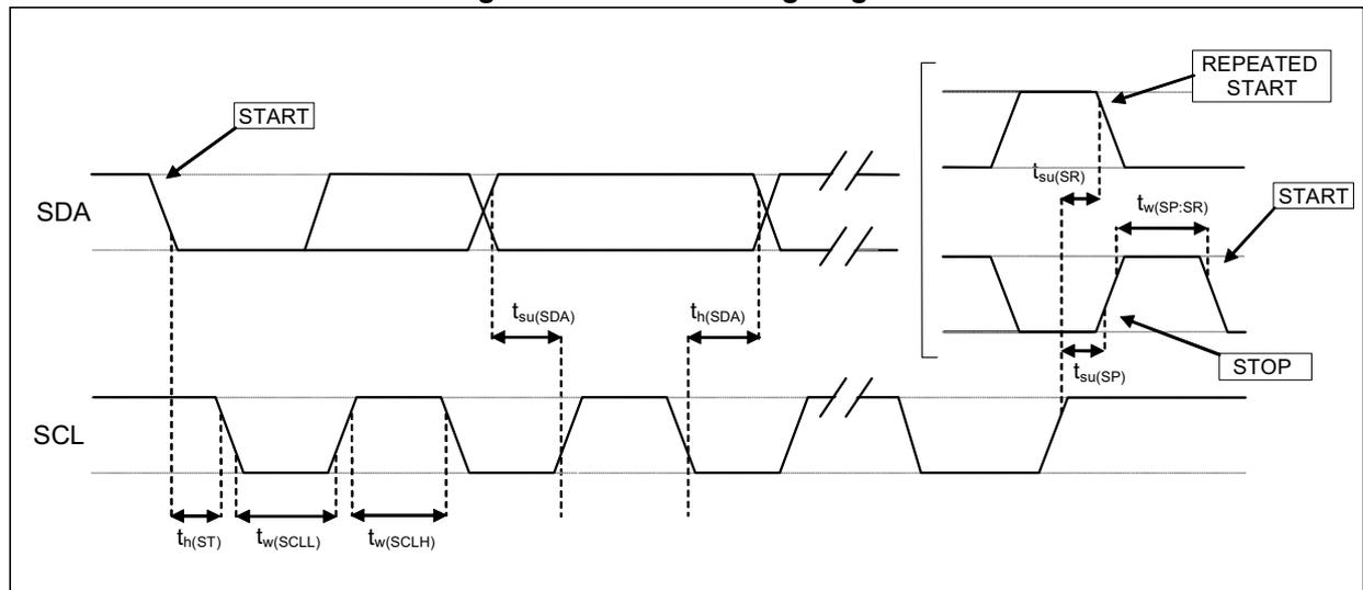
Note: Measurement points are done at 0.2·V<sub>DD\_IO</sub> and 0.8·V<sub>DD\_IO</sub>, for both ports.
