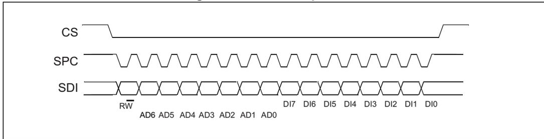
The SPI write command is performed with 16 clock pulses. The multiple byte write command is performed by adding blocks of 8 clock pulses to the previous one.
