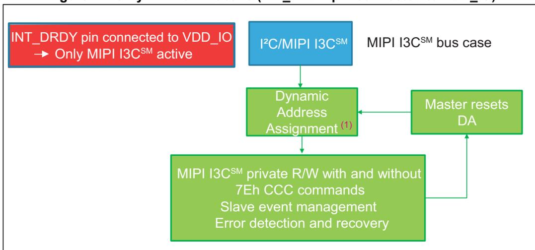
1. When the slave is MIPI I3C<sup>SM</sup> only, the I<sup>2</sup>C slave is always disabled. The address can be assigned using MIPI I3C<sup>SM</sup> SDR timing.
