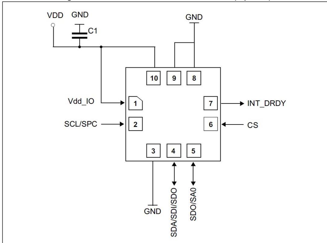
The device power supply must be provided through the VDD line; a power supply decoupling capacitor C1 (100 nF) must be placed as near as possible to the supply pads of the device. The C1 capacitor can be tied to VDD and VDDIO, but it is recommended to use 2 capacitors, one on each VDD and VDDIO line, in case VDD and VDDIO are separate. Depending on the application, an additional capacitor of 4.7  $\mu$ F could be placed on VDD line.
