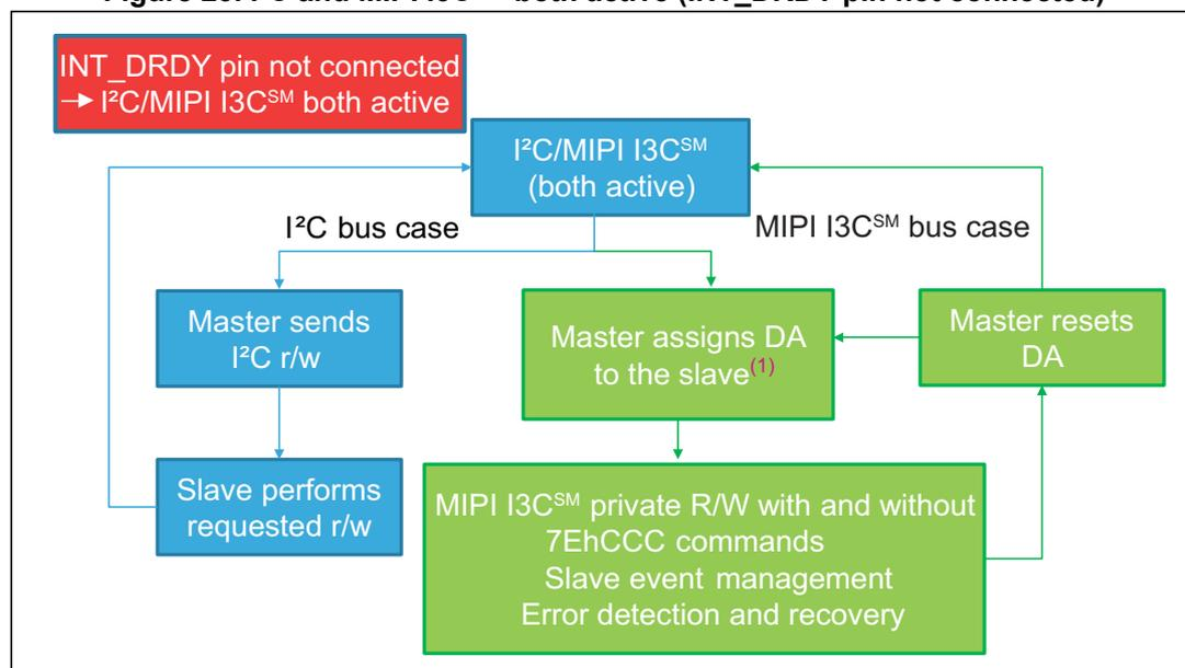
1. Address assignment (SETDASA) must be performed with I<sup>2</sup>C Fast Mode Plus Timing. When the slave is addressed, the I<sup>2</sup>C slave is disabled and the timing is compatible with MIPI I3C<sup>SM</sup> specifications.
