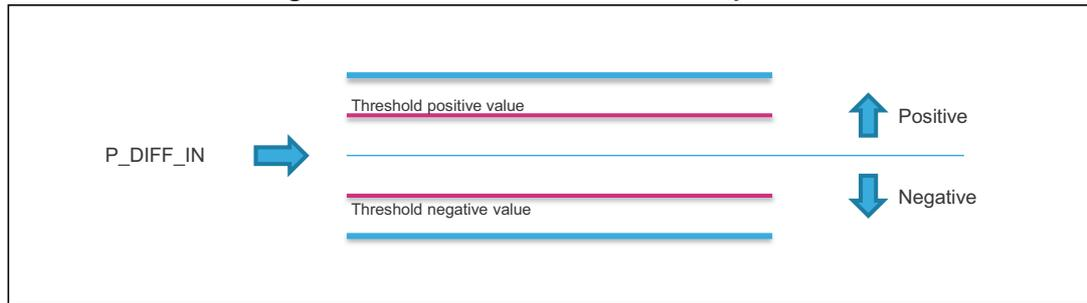
To enable the **AUTOZERO** mode, the AUTOZERO bit must be set to '1' and then the measured pressure value is used as the reference and stored in the register REF\_P (*REF\_P\_L (15h)*, *REF\_P\_H (16h)*). From this point on, the output pressure value (*PRESS\_OUT\_XL (28h)*, *PRESS\_OUT\_L (29h)*, *PRESS\_OUT\_H (2Ah)*) is updated with the difference between the measured pressure and REF\_P.
