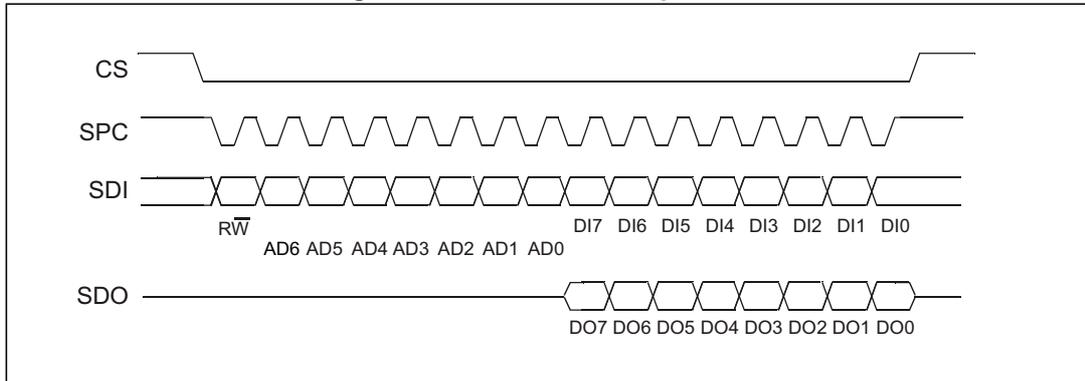
**CS** is the serial port enable and it is controlled by the SPI master. It goes low at the start of the transmission and returns to high at the end. **SPC** is the serial port clock and it is controlled by the SPI master. It is stopped high when **CS** is high (no transmission). **SDI** and **SDO** are respectively the serial port data input and output. Those lines are driven at the falling edge of **SPC** and should be captured at the rising edge of **SPC**.
