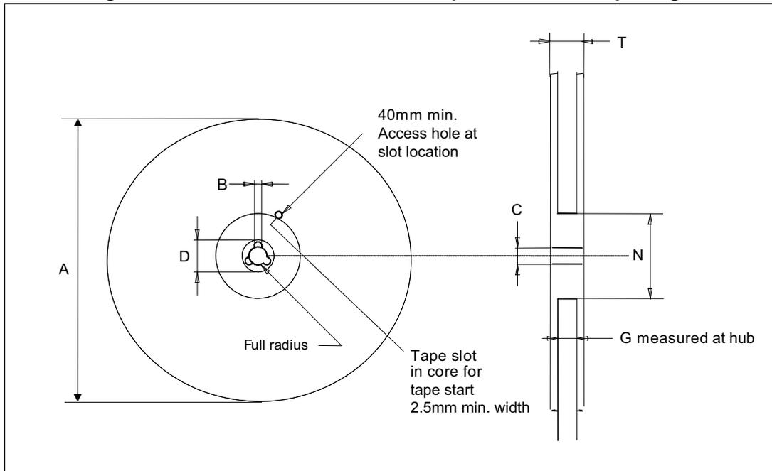
Table 24. Reel dimensions for carrier tape of CCLGA-10L package
