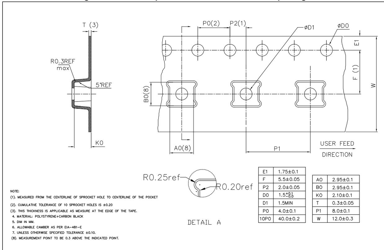
Figure 29. Package orientation in carrier tape
