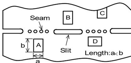
\*1 A > D is valid when stress is added vertically to the perforation as with Hand Separation. If a Cutting Disc is used, stress will be diagonal to the PCB, therefore A > D is invalid.
