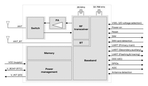
Figure 2: SARA-N3 series block diagram
