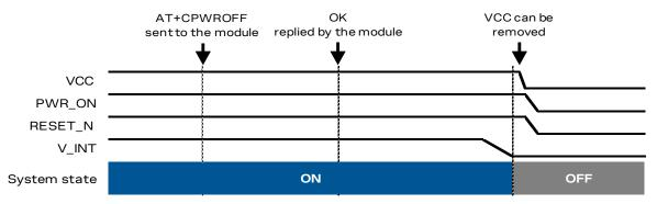
Figure 10: SARA-N3 series modules switch-off sequence by means of AT+CPWROFF command
