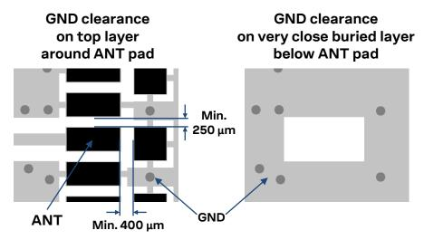
Figure 24: GND keep-out area on the top layer around ANT pad and on the very close buried layer below ANT pad
