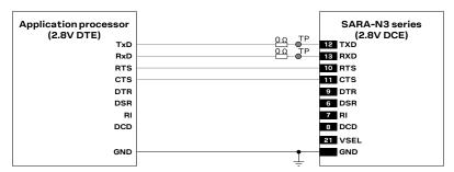
Figure 36: SARA-N3 series' UART application circuit with TXD, RXD, RTS and CTS lines connection (2.8 V DTE / 2.8 V DCE)
