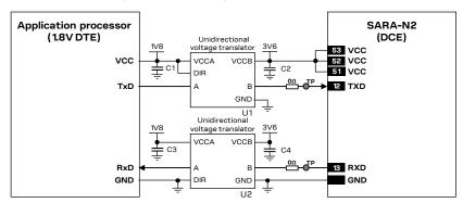
Figure 40: SARA-N2 series' UART interface application circuit with TXD and RXD lines connection to 1.8 V DTE
