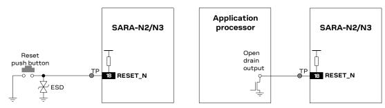
Figure 21: RESET\_N application circuits using a push button and an open drain output of an application processor
