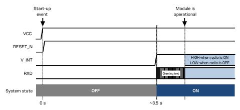
Figure 8: SARA-N2 series power-on sequence from not-powered mode
