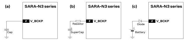
Figure 19: V\_BCKP application circuits using: (a) a capacitor, (b) a supercapacitor, (c) a non-rechargeable battery
