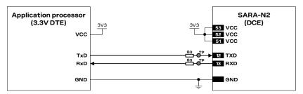
Figure 39: SARA-N2 series' UART interface application circuit with TXD and RXD lines connection to 3.3 V DTE
