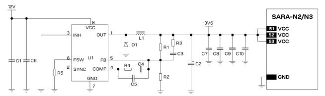
Figure 16: Suggested schematic design for the VCC voltage supply application circuit using a step-down regulator
