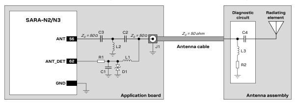
Figure 28: Suggested schematic for antenna detection circuit on application PCB and diagnostic circuit on antenna assembly
