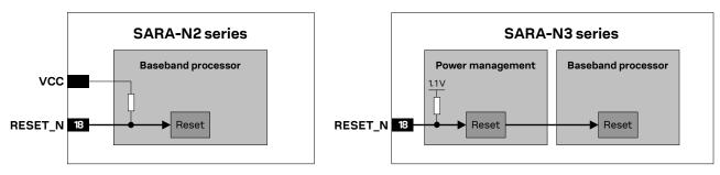
Figure 11: SARA-N2 / N3 series RESET\_N input equivalent circuit description
