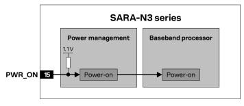
Figure 7: SARA-N3 series PWR\_ON input equivalent circuit description
