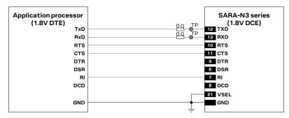
Figure 33: SARA-N3 series' UART application circuit with TXD, RXD, RTS, CTS and RI lines connection (1.8 V DTE / 1.8 V DCE)
