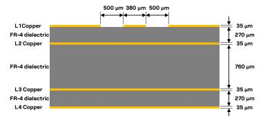
Figure 25: Example of  $50 \Omega$  coplanar waveguide transmission line design for the described 4-layer board layup
