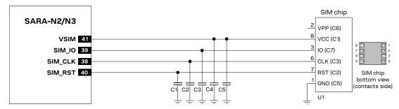
Figure 31: Application circuit for the connection to a single solderable SIM chip
