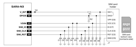
Figure 32: Application circuit for the connection to a single removable SIM card, with SIM detection implemented
