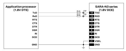
Figure 37: SARA-N3 series' UART application circuit with TXD and RXD lines connection (1.8 V DTE / 1.8 V DCE)
