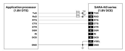
Figure 35: SARA-N3 series' UART application circuit with TXD, RXD, RTS and CTS lines connection (1.8 V DTE / 1.8 V DCE)
