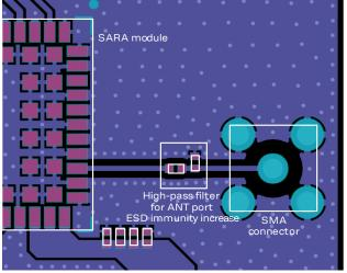
Figure 27: Suggested circuit and layout for antenna RF circuit on application board, if antenna detection is not required
