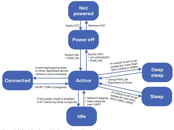
Figure 4: SARA-N3 series modules' operating modes transitions
