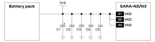
Figure 14: Suggested schematic design for the VCC voltage supply application circuit using a LiSOCl<sub>2</sub> primary battery
