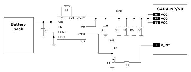
Figure 15: Alternative schematic design for the VCC voltage supply application circuit using a generic primary battery
