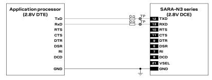
Figure 38: SARA-N3 series' UART application circuit with TXD and RXD lines connection (2.8 V DTE / 2.8 V DCE)
