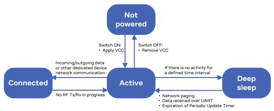
Figure 3: SARA-N2 series modules' operating modes transitions
