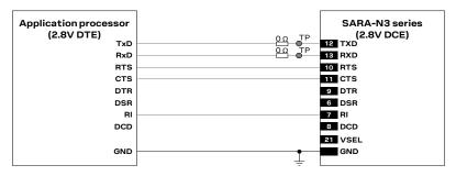
Figure 34: SARA-N3 series' UART application circuit with TXD, RXD, RTS, CTS and RI lines connection (2.8 V DTE / 2.8 V DCE)
