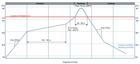
Figure 51: Recommended soldering profile
