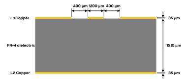
Figure 26: Example of  $50\,\Omega$  coplanar waveguide transmission line design for the described 2-layer board layup
