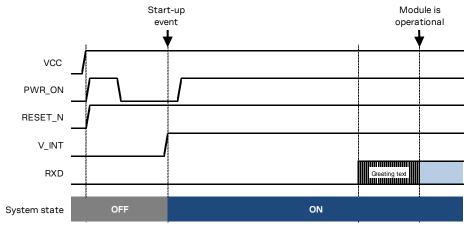
Figure 9: SARA-N3 series power-on sequence from not-powered mode
