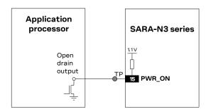
Figure 20: PWR\_ON application circuits using a push button and an open drain output of an application processor
