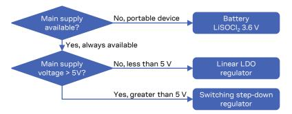
Figure 13: VCC supply concept selection
