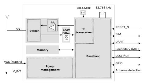
Figure 1: SARA-N2 series modules block diagram
