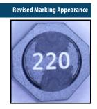
The form of the inductor will change due to the change in the marking method. The fit and function will remain the same. The quality and reliability should be improved as the result of the manufacturing process change.
