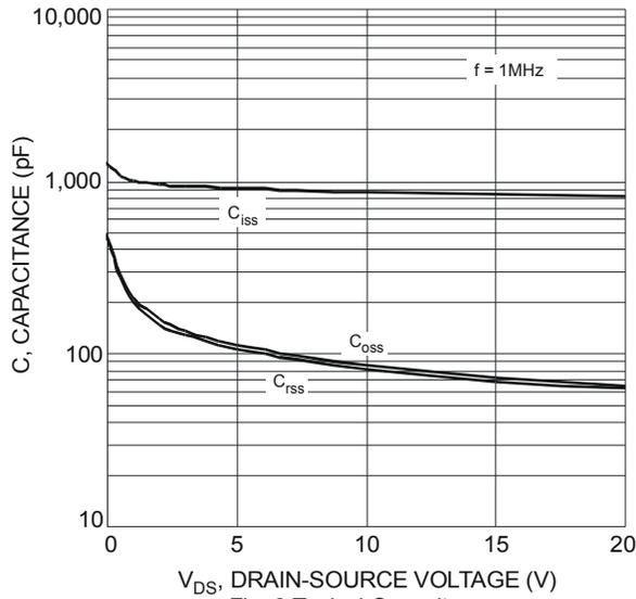
Fig. 9 Typical Capacitance
