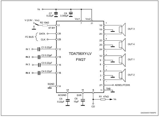
Figure 2. Application circuit
