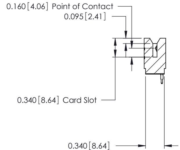
746 Series Ultra-Mate Card Edge Connector - Press Fit
