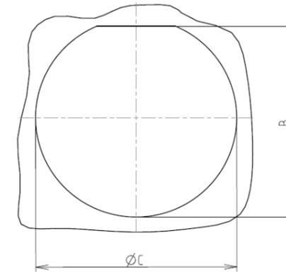
Max. thickness panel for receptacle: Type 7: 3.2 mm
