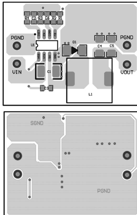
**Figure 7: PCB Layout**
