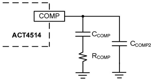
①: C<sub>COMP2</sub> is needed only for high ESR output capacitor
