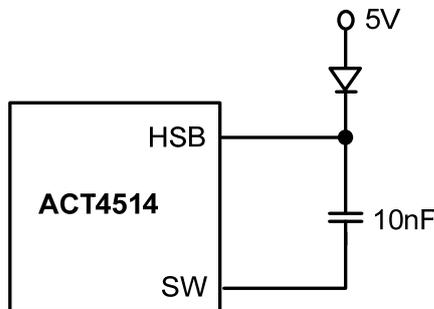
This diode is also recommended for high duty cycle operation and high output voltage applications.
