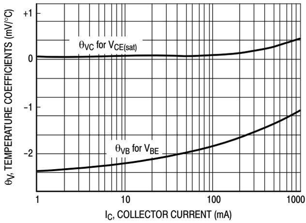
Figure 4. Temperature Coefficients
