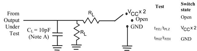
FIGURE 3. AC Loading Circuit for LVTTTL Outputs
