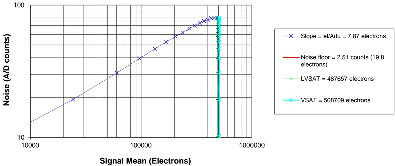
Figure 3. Measured Performance – Dynamic Range and Noise Floor
