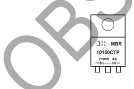
MBR10150CTP = Product Type Marking Code AB = Foundry and Assembly Code YYWW = Date Code Marking YY = Last two digits of year (ex: 08 = 2008) WW = Week (01 - 53)
