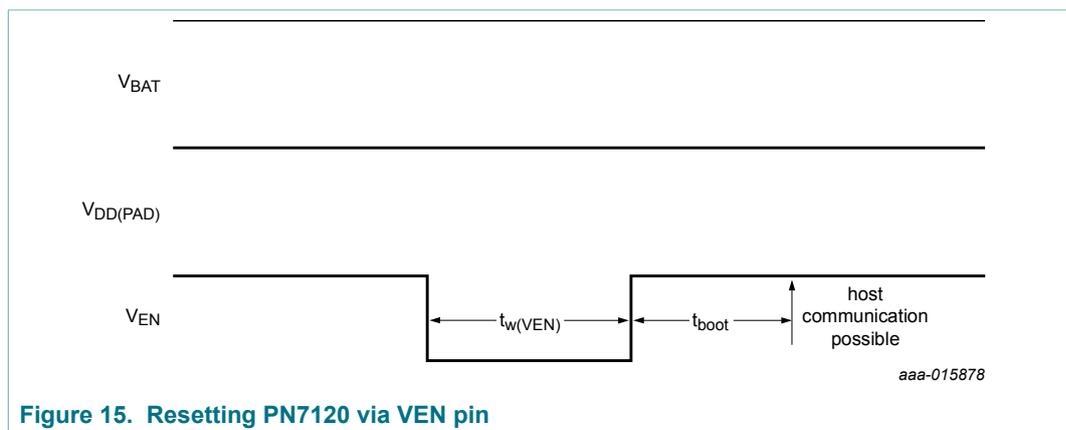
Figure 15. Resetting PN7120 via VEN pin
