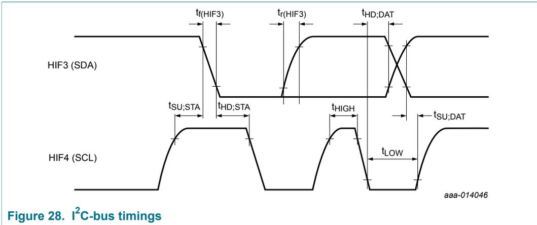
Figure 28. I<sup>2</sup>C-bus timings
