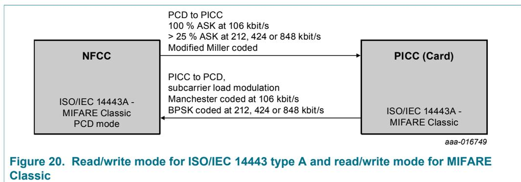
**Figure 20. Read/write mode for ISO/IEC 14443 type A and read/write mode for MIFARE Classic**
