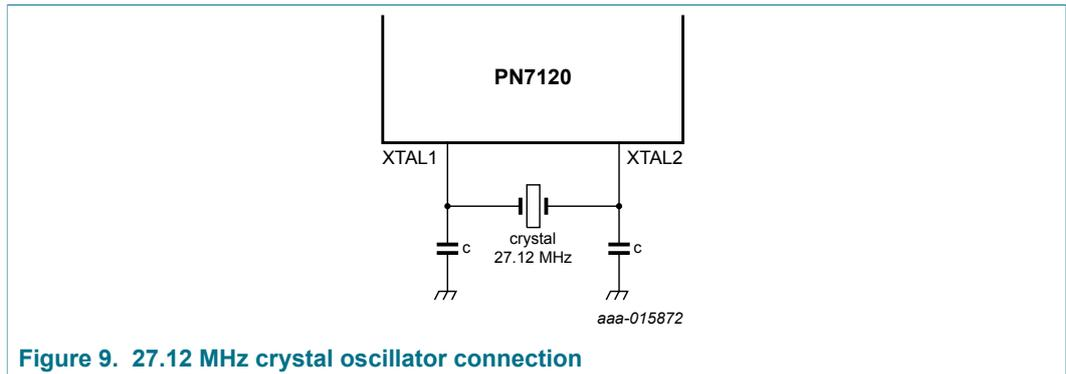
Figure 9. 27.12 MHz crystal oscillator connection
