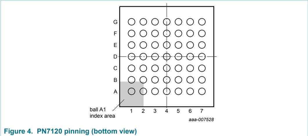
Figure 4. PN7120 pinning (bottom view)
