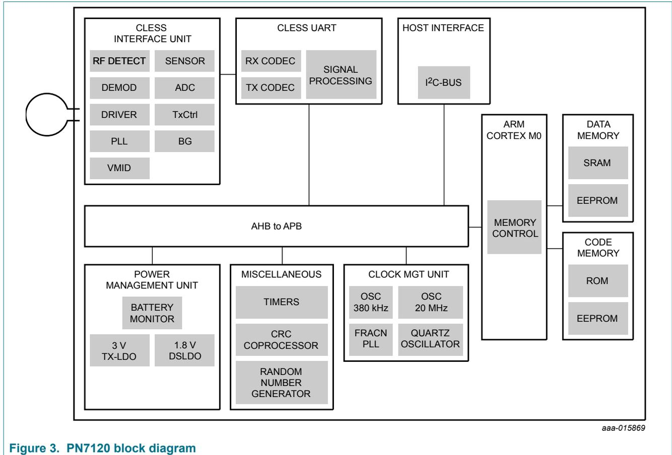
Figure 3. PN7120 block diagram
