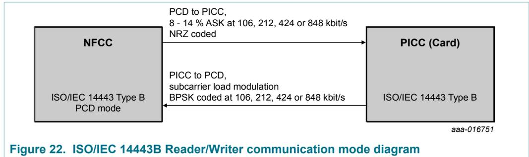
Figure 22. ISO/IEC 14443B Reader/Writer communication mode diagram
