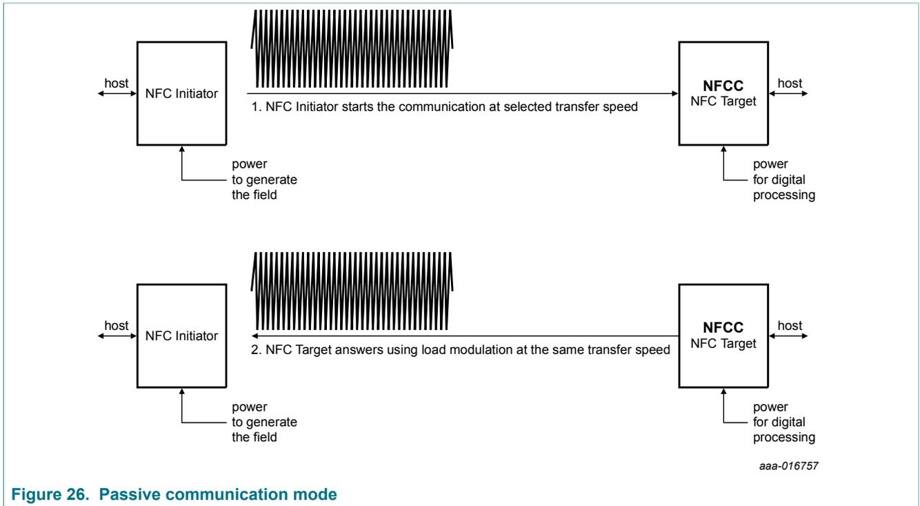
Figure 26. Passive communication mode
