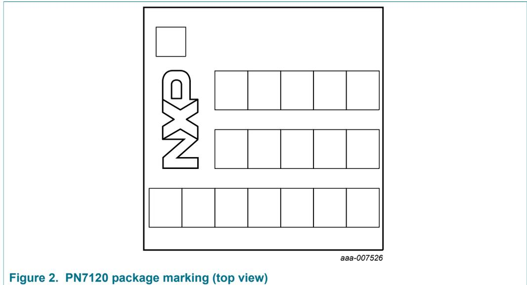
Figure 2. PN7120 package marking (top view)
