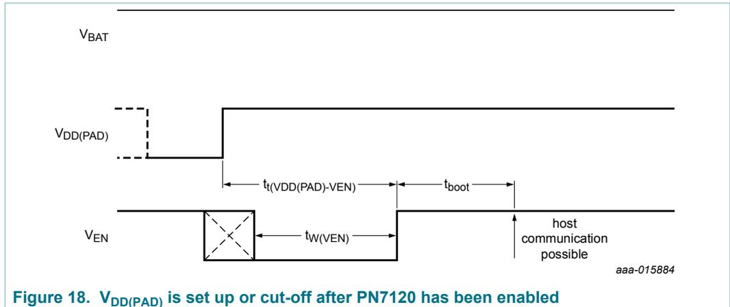
Figure 18. V<sub>DD(PAD)</sub> is set up or cut-off after PN7120 has been enabled
