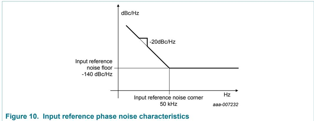
Figure 10. Input reference phase noise characteristics
