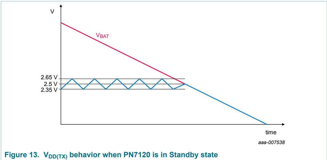
Figure 13.  $V_{DD(TX)}$  behavior when PN7120 is in Standby state
