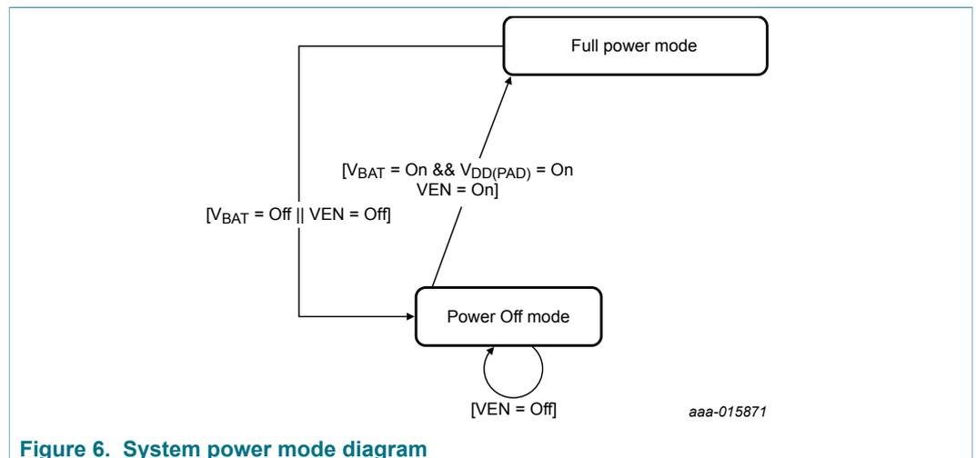
**Figure 6. System power mode diagram**
