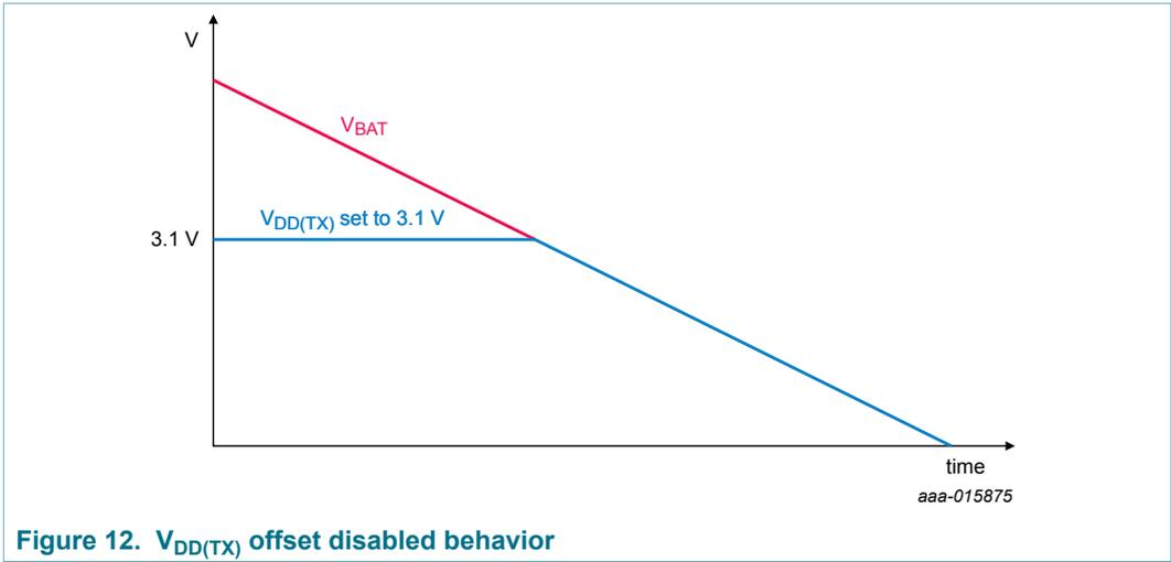
Figure 12.  $V_{DD(TX)}$  offset disabled behavior
