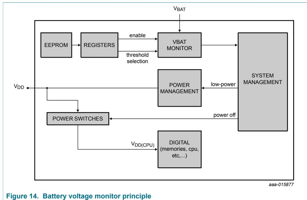
Figure 14. Battery voltage monitor principle
