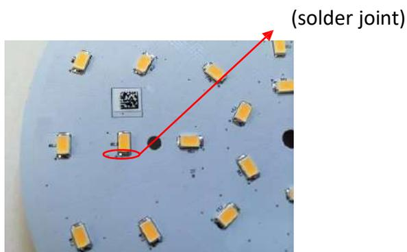
You can use the high-temperature thermal conductivity glue (Such as SatlonD-3/606...etc.) to fix the thermal couple to the solder joint then measure the temperature. Once you got the  $T_s$  temperature measurement data, you can calculate the junction temperature based on the measurement data of the  $T_s$ . The details of the calculation method are shown in the following page:
