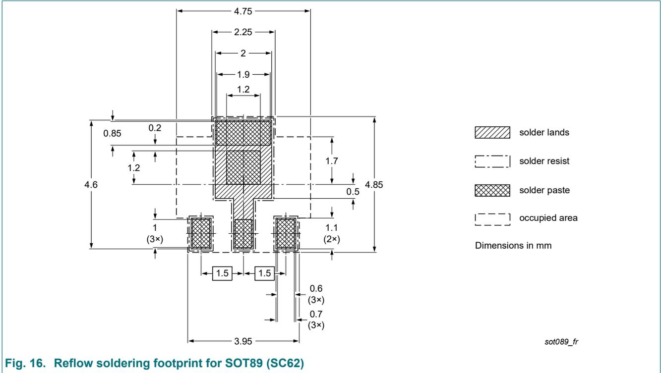
Fig. 16. Reflow soldering footprint for SOT89 (SC62)
