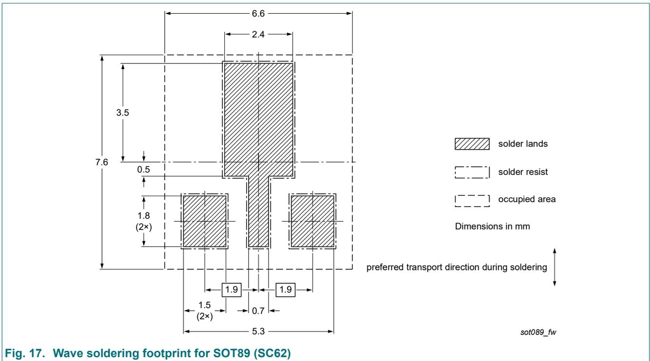
Fig. 17. Wave soldering footprint for SOT89 (SC62)
