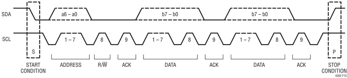
Figure 15. Data Transfer Over I<sup>2</sup>C or SMBus
