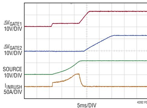
Figure 8. Start-Up Waveform
