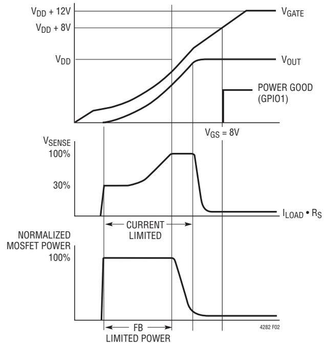
Figure 2. Power-Up Waveforms
