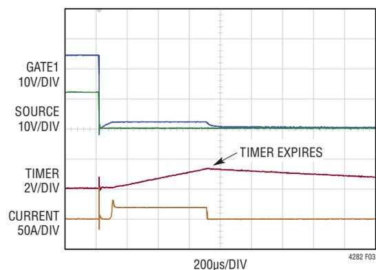
Figure 3. Short-Circuit Waveform
