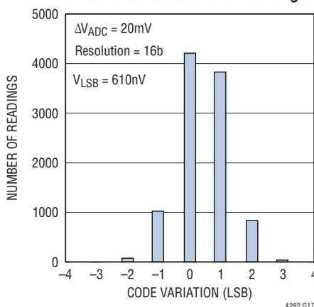
**12 Bit GPIO ADC Noise Histogram**
