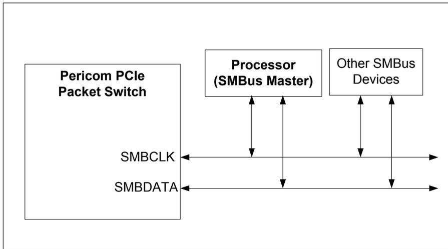
The SMBus interface on the Packet Switch consists of one SMBus clock pin (SCL\_I2C), a SMBus data pin (SDA\_I2C), and 3 SMBus address pins (GPIO[7:5]). The SMBus clock pin provides or receives the clock signal. The SMBus data pin facilitates the data transmission and reception. Both of the clock and data pins are bi-directional. The SMBus address pins determine the address to which the Packet Switch responds to. The SMBus address pins generate addresses according to the following table:
