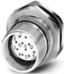
Device connector for rear wall, straight, shielded: yes, SPEEDCON locking, M23, Number of positions: 12, Type of contact: Socket, Crimp connection, Seal, axial, Central fixing
