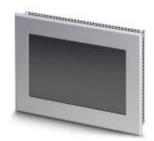
Touch panel with 17.8 cm/7" TFT-Display (Analog resistive (polyester)), 800 x 480 Pixel (WVGA), 262144 colors, ARM® Cortex®-A8, 800 MHz, 2x USB host 2.0, 1 x Ethernet (10/100 Mbps), RJ45, Windows® Embedded Compact 7 and User software: IniNet Browser. (Bus system: without)
