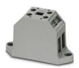
Device terminal block, Connection method: Screw connection, Number of positions: 2, Cross section: 0.5 mm² - 16 mm², AWG: 20 - 6, Width: 24.8 mm, Height: 40 mm, Color: gray, Mounting type: Screw mounting
