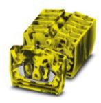
Mini feed-through terminal block, Connection method: Spring-cage connection, Cross section: 0.08 mm² - 4 mm², AWG: 28 - 12, Width: 5.2 mm, Height: 22 mm, Color: black/yellow, Mounting type: Direct mounting with flange
