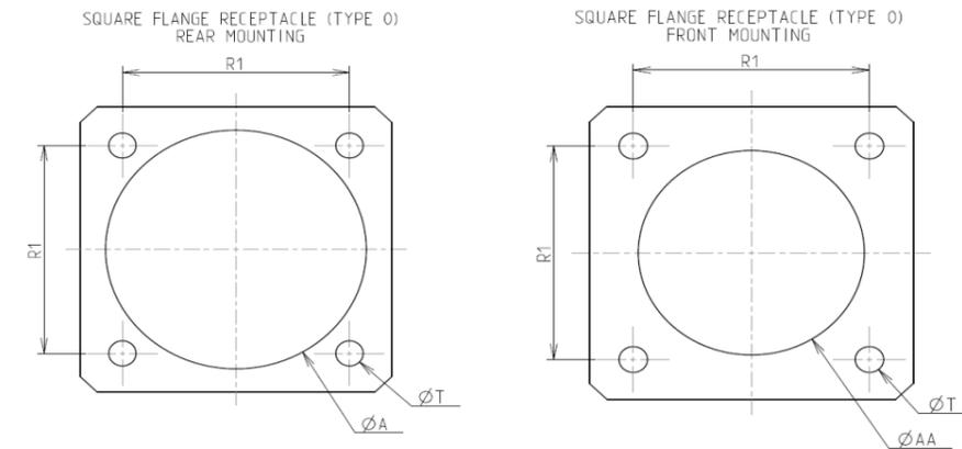
Max. thickness panel for receptacle: Type 0: front mounting = 3.2 mm, rear mounting = 2.5 mm
