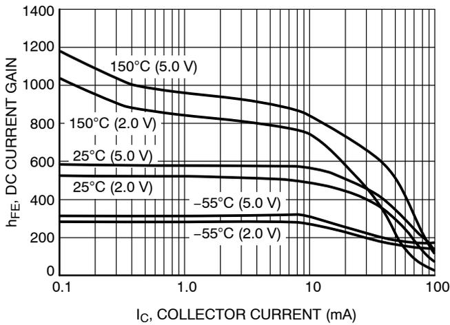
Figure 3. DC Current Gain vs. Collector Current
