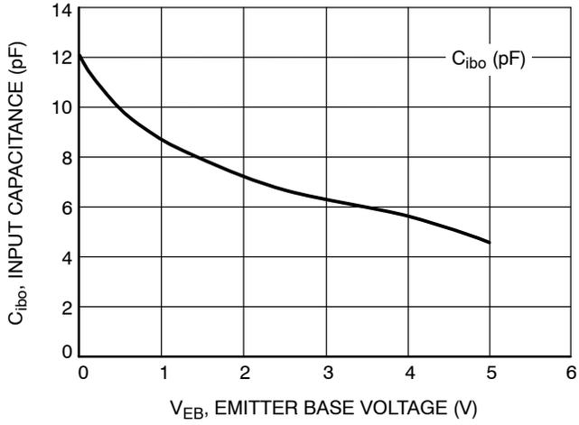
Figure 7. Input Capacitance
