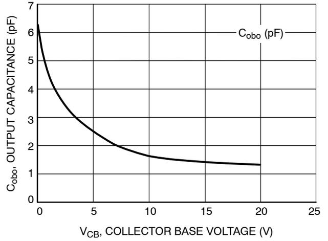
Figure 8. Output Capacitance
