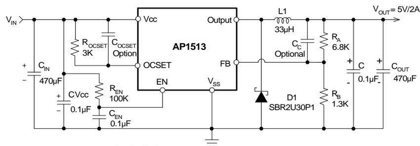
Note:  $V_{OUT} = V_{FB} \times (1 + R_A/R_B)$
