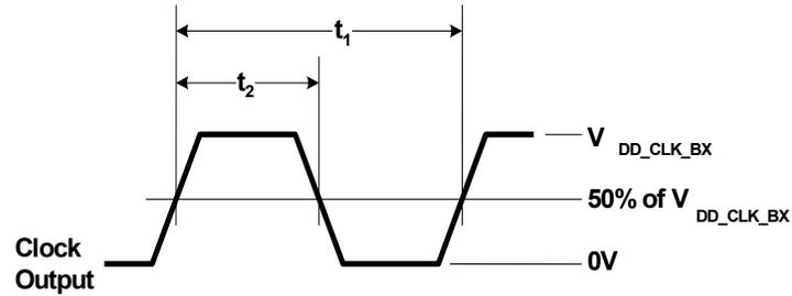
**Figure 9. Rise Time =  $T_{RF}$ , Fall Time =  $T_{RF}$**
