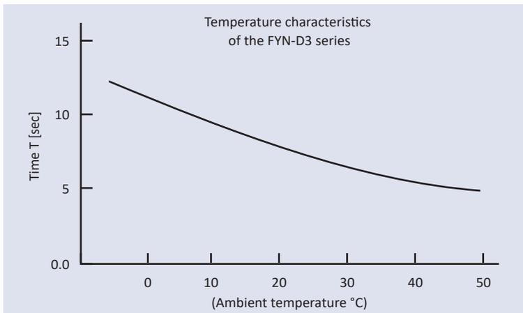
■ Damper characteristics vary according to the ambient temperature. In general, the damper characteristics become weaker as the temperature increases, and become stronger as the temperature decreases. This is because the viscosity of the oil inside the damper varies according to the temperature. When the temperature returns to normal, the damper characteristics will return to normal as well. The changes in the time it takes for the lid to close are shown in the graph to the left.
