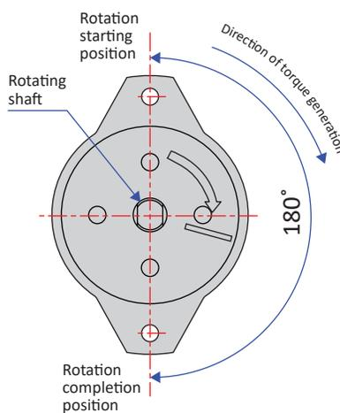
The damper's working angle is 180° with respect to the attachment flange, as shown to the left. Please determine where to attach it according to your needs. Also, rotating the damper beyond this angle will cause damage to the damper. Please ensure that an external stopper is in place.
