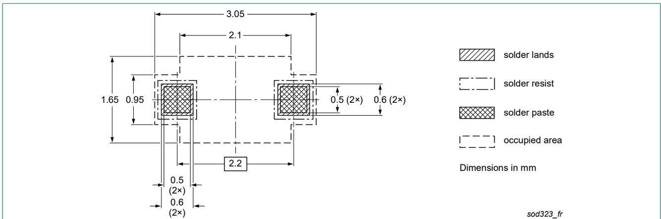
Fig. 6. Reflow soldering footprint for SOD323
