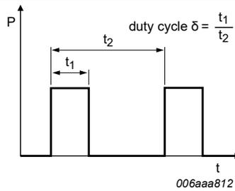
Fig. 4. Duty cycle definition
