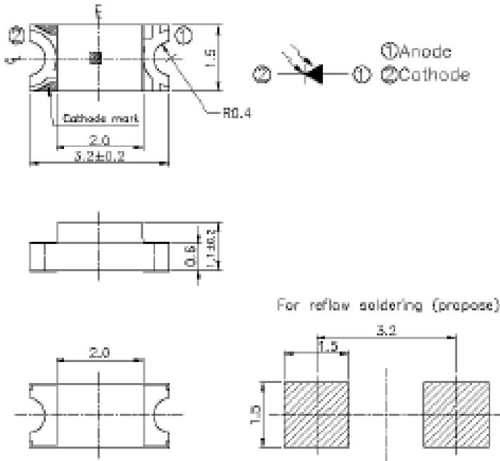
>Soldering Conditions: 260°C 1/16 inch away from case for 3 seconds max.
