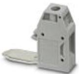
Pick-off terminal block, Connection method: Screw connection, Cross section: 0.5 mm<sup>2</sup> - 10 mm<sup>2</sup>, AWG: 20 - 8, Width: 10.2 mm, Height: 34.7 mm, Color: gray, Mounting type: On base element
