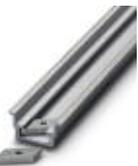
DIN rail, deep drawn, high profile, unperforated, 1.5 mm thick, material: aluminum, height 15 mm, width 35 mm, length 2000 mm
