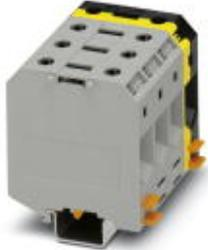
High-current terminal block, Connection method: Screw connection, Number of positions: 4, Cross section: 16 mm<sup>2</sup> - 70 mm<sup>2</sup>, AWG: 6 - 2/0, Width: 80 mm, Color: gray/black-yellow, Mounting type: NS 35/7,5, NS 35/15, NS 32, NS 35/15-2,3
