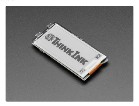
Easy e-paper finally comes to Raspberry Pi, with this bonnet that's designed to make it a breeze to add a 2.13" 250x122 crisp monochromic elnk display. Chances are you've seen one of those new-fangled 'e-readers' like the Kindle or Nook. They have gigantic electronic paper 'static' displays - that means the image stays on the display even when power is completely disconnected. The image is also high contrast and very daylight readable. It really does look just like printed paper!
