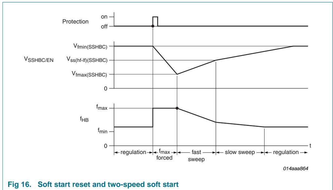
**Fig 16. Soft start reset and two-speed soft start**
