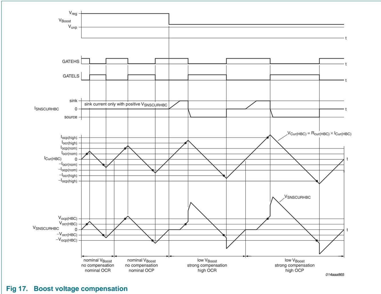
Fig 17. Boost voltage compensation
