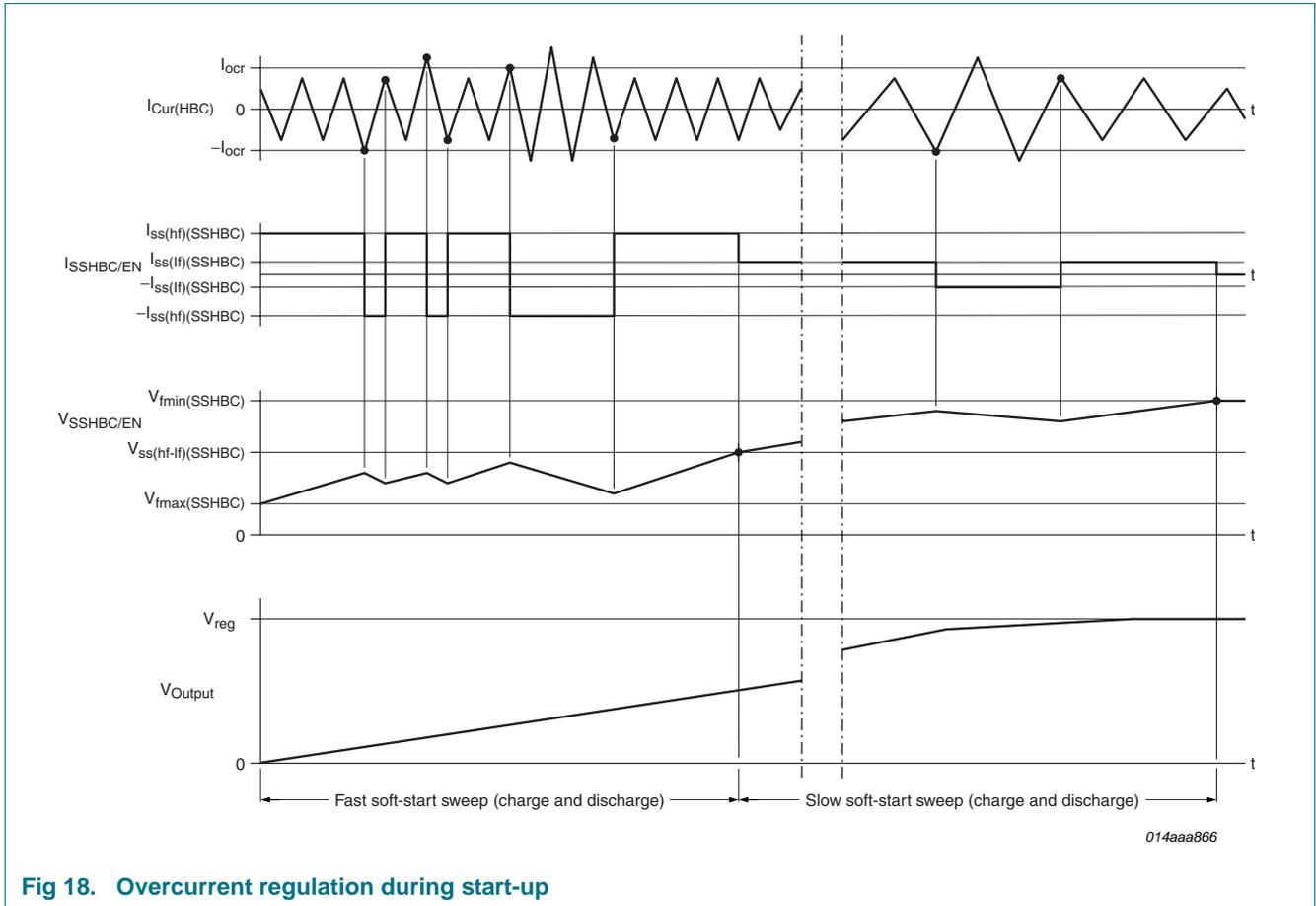
Fig 18. Overcurrent regulation during start-up
