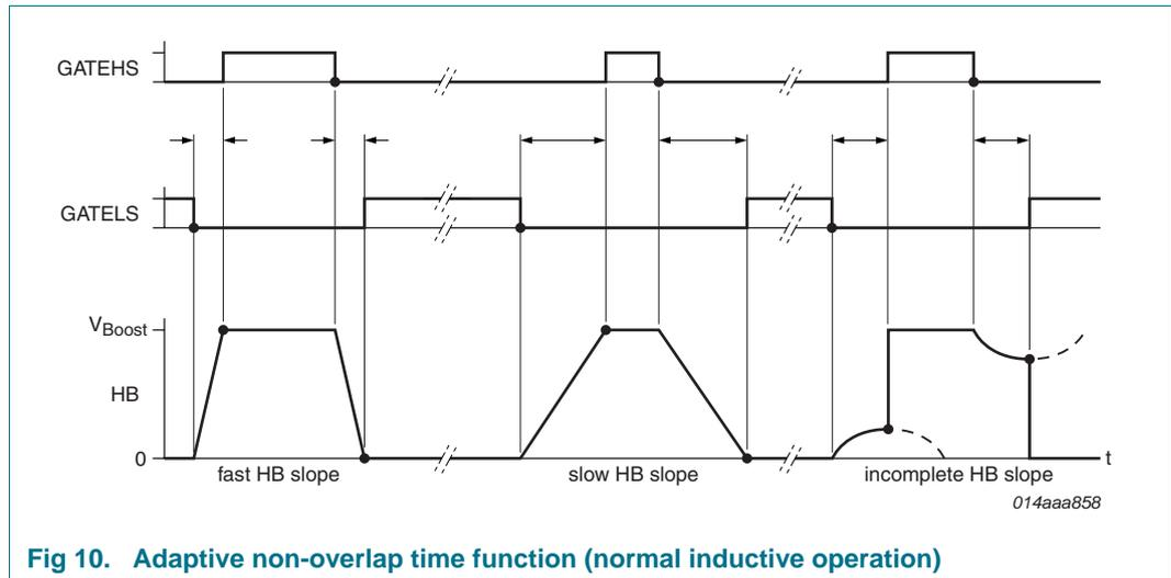
**Fig 10. Adaptive non-overlap time function (normal inductive operation)**
