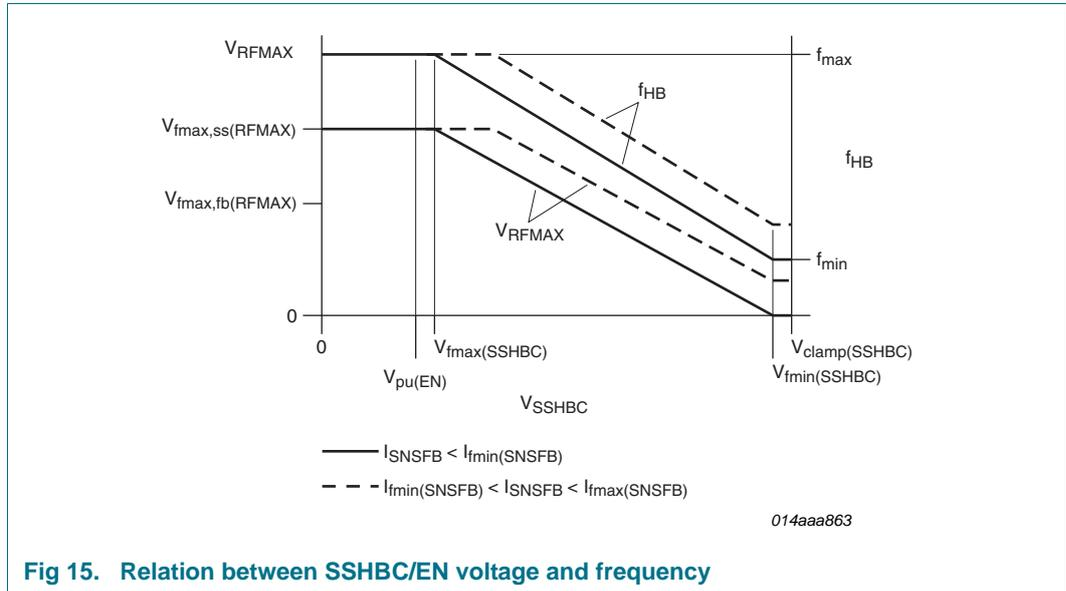
Fig 15. Relation between SSHBC/EN voltage and frequency
