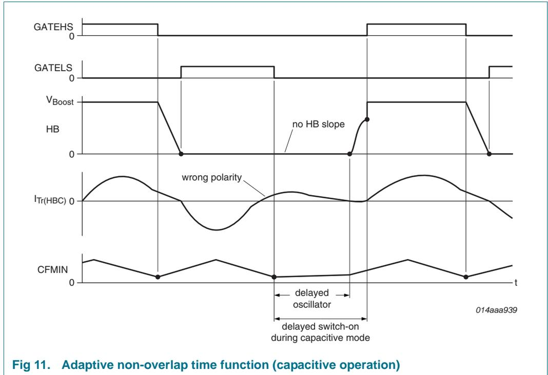
**Fig 11. Adaptive non-overlap time function (capacitive operation)**
