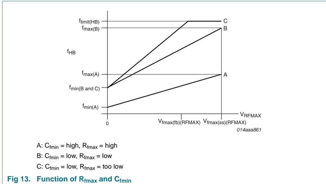
Fig 13. Function of  $R_{fmax}$  and  $C_{fmin}$
