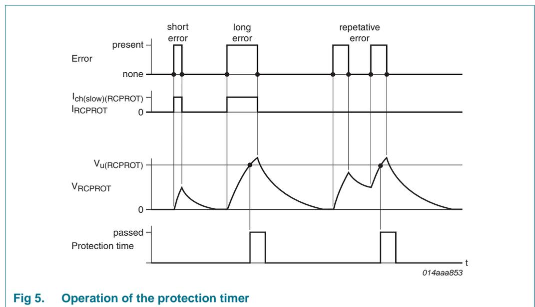
**Fig 5. Operation of the protection timer**
