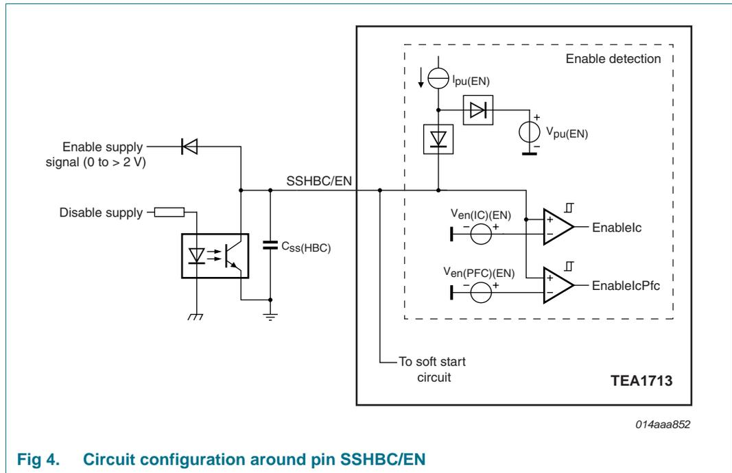
Fig 4. Circuit configuration around pin SSHBC/EN
