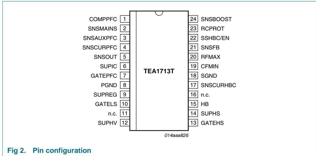
Fig 2. Pin configuration
