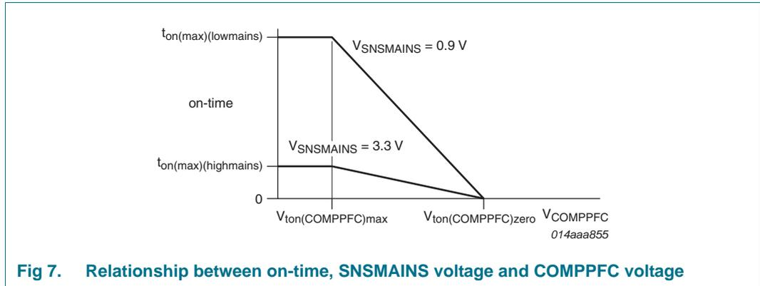
Fig 7. Relationship between on-time, SNSMAINS voltage and COMPPFC voltage
