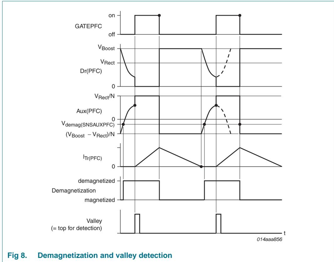
Fig 8. Demagnetization and valley detection
