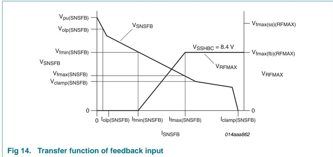
Fig 14. Transfer function of feedback input
