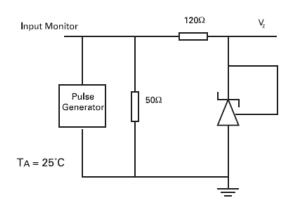
**Test Circuit for Pulse Response**
