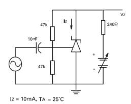
Test Circuit for Open Loop Voltage Gain
