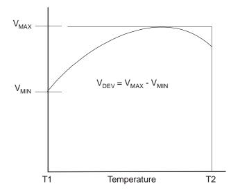
$$V_{ref} (ppm/^{o} C) = \frac{V_{dev} \times 1000000}{V_{ref} (T1 - T2)}$$
