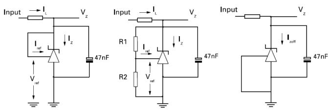
Figure 1. Test Circuit for  $V_Z = V_{REF}$
