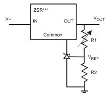
$V_{OUT(MIN)} = V_{REF} + V_{REG}$
