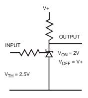
SINGLE SUPPLY COMPARATOR WITH TEMPERATURE COMPENSATED THRESHOLD
