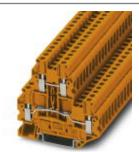
Double-level terminal block, connection method: Screw connection, cross section: 0.14 mm² - 4 mm², AWG: 26 - 12, width: 5.2 mm, color: orange, mounting type: NS 35/7,5, NS 35/15
