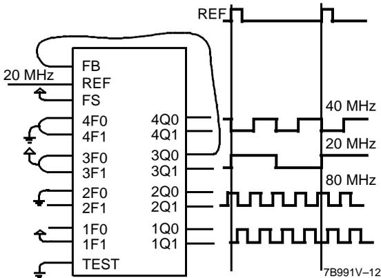
Figure 6 shows the LVPSCB configured as a clock multiplier. The 3Q0 output is programmed to divide by four and is sent back to FB. This causes the PLL to increase its frequency until the 3Q0 and 3Q1 outputs are locked at 20 MHz, while the 1Qx and 2Qx outputs run at 80 MHz. The 4Q0 and 4Q1 outputs are programmed to divide by two that results in a 40 MHz waveform at these outputs. Note that the 20- and 40-MHz clocks fall
